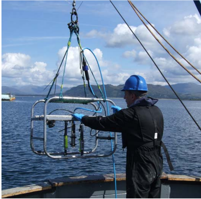
Figure 9 –The camera being deployed (Dunstaffnage site) over the stern of the RV Seol Mara. Note the downward facing, parallel mounted torches (yellow) on the camera frame.
