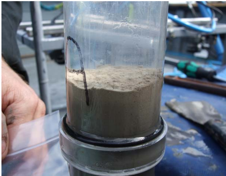
Figure 11 – A typical core from a non-impacted part of the Dunstaffnage site. The top 10 mm was removed for sedimentary analysis (LOI250 and 500 and particle size analysis).
