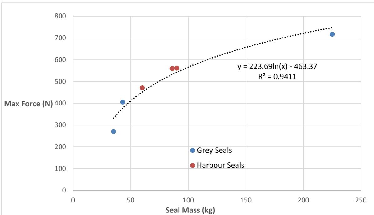
Figure 15 - Seal mass vs maximum force output
