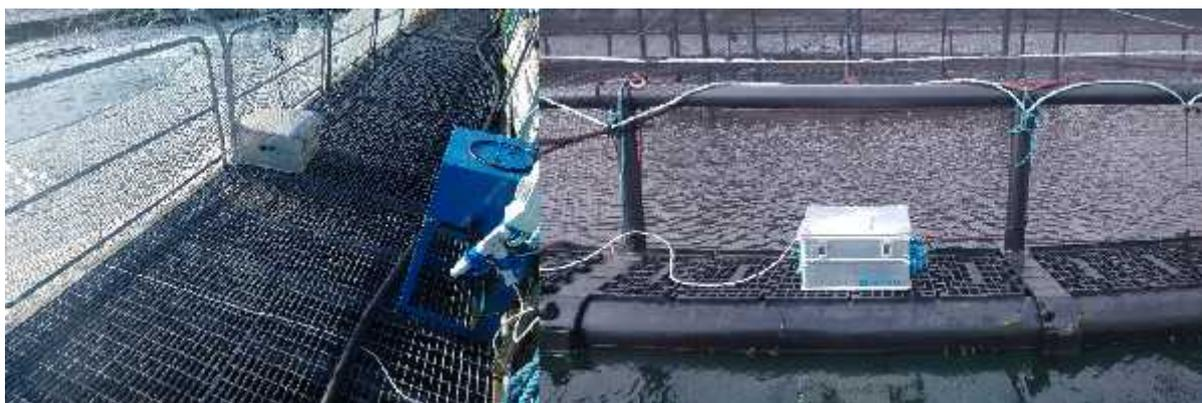
Figure 6 - Deployments of recorder on steel walkway and plastic circles
