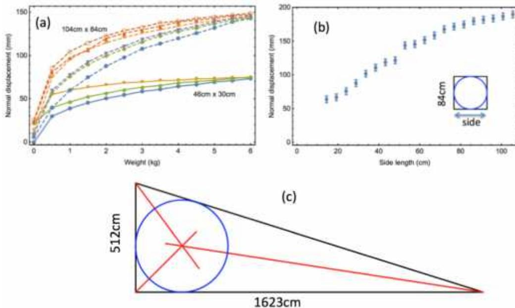
Figure 17 - (a) Measured net displacement vs weight for two frame sizes, (b) Net deflection vs length of panel side, (c) Geometry used to calculate the point of maximal deflection
