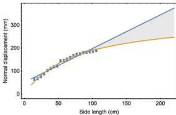
Figure 18 - Linear and logarithmic extrapolations of net deformation vs net size
