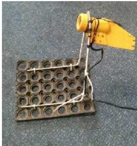
Figure 5 - Underwater camera attached to mounting frame
