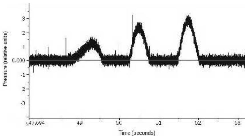
Figure 13 - High frequency force measurements, showing the impulsive nature of the seal attacks. Amplitude increases until the seal is able to reach the target and receive the reward.
